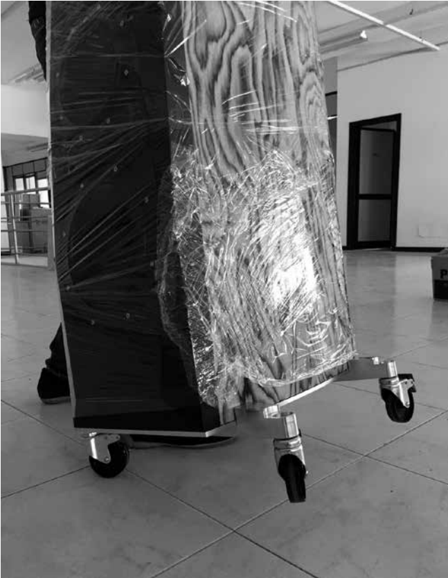
When in place, activate brakes on all wheels and tilt speaker pivoting it on a side wheel pair. Two or more people needed.
