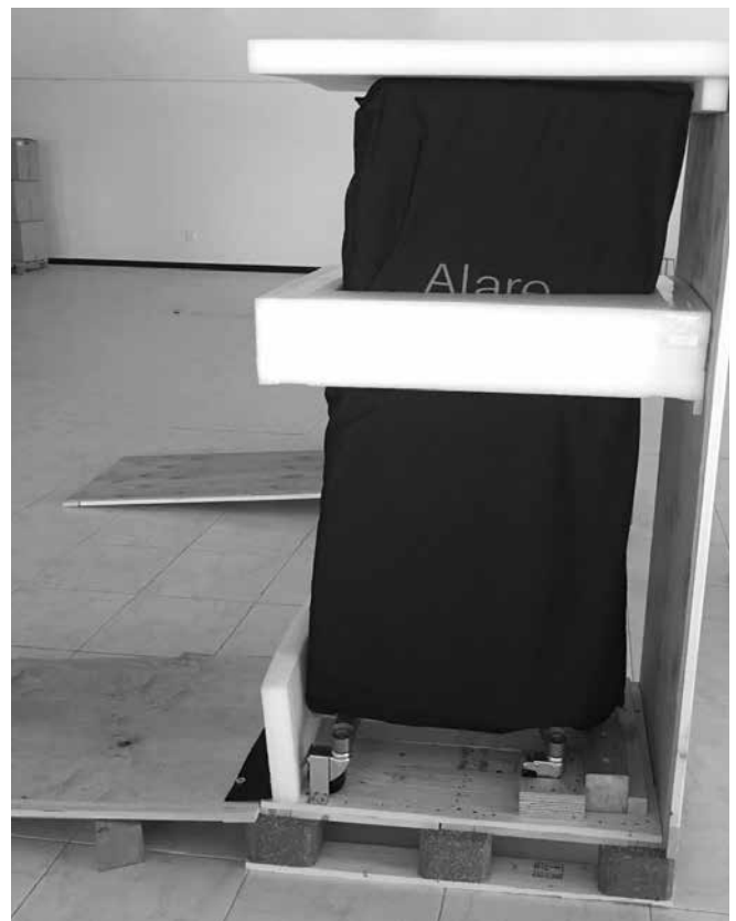
Remove side and rear panels and foam pads. Attention, wooden panels are free when clamps are removed.
