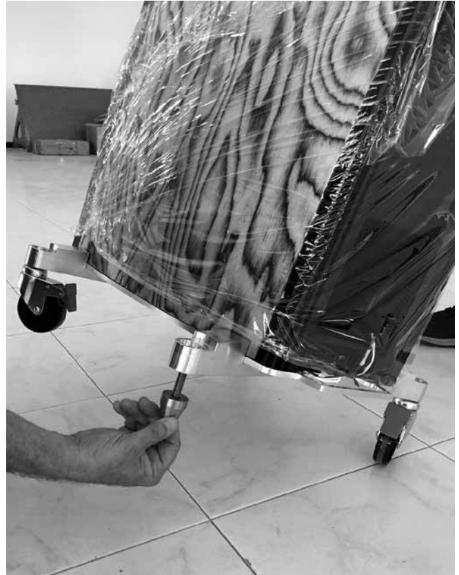
Unscrew the floating pair of wheels and substitute them with spikes at maximum thread length. Repeat this procedure on the other side.
